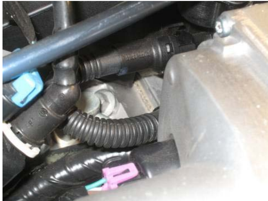
Figure 4: PCV Line Intake Plenum Connection
