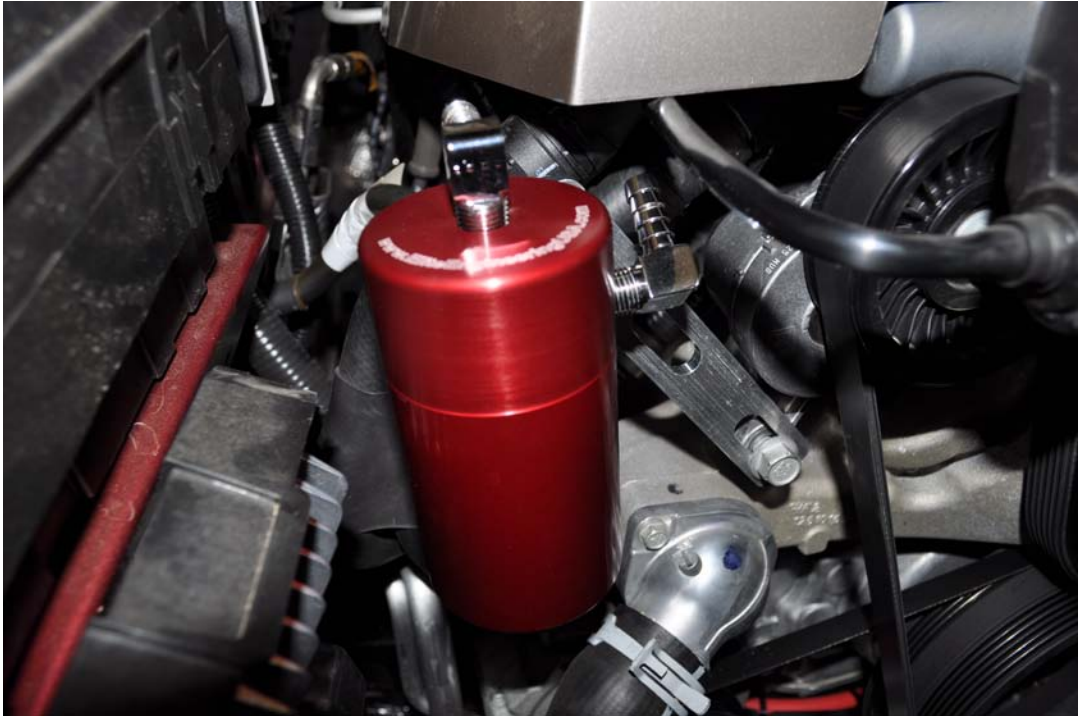
Figure 7: Catch Can Installed on Bracket
