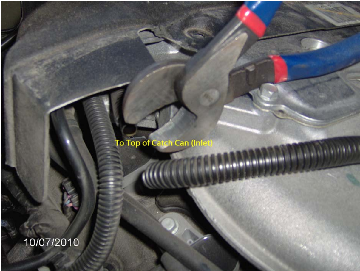
Figure 2: Cut Vacuum Line
